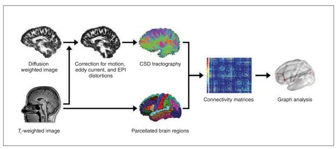
Fig. 1: Flowchart of the preprocessing pipeline using FreeSurfer (https://surfer.nmr.mgh.harvard.edu) and ExploreDTI (www.exploredti.com). CSD = constrained spherical deconvolution; EPI = echo-planar imaging.
